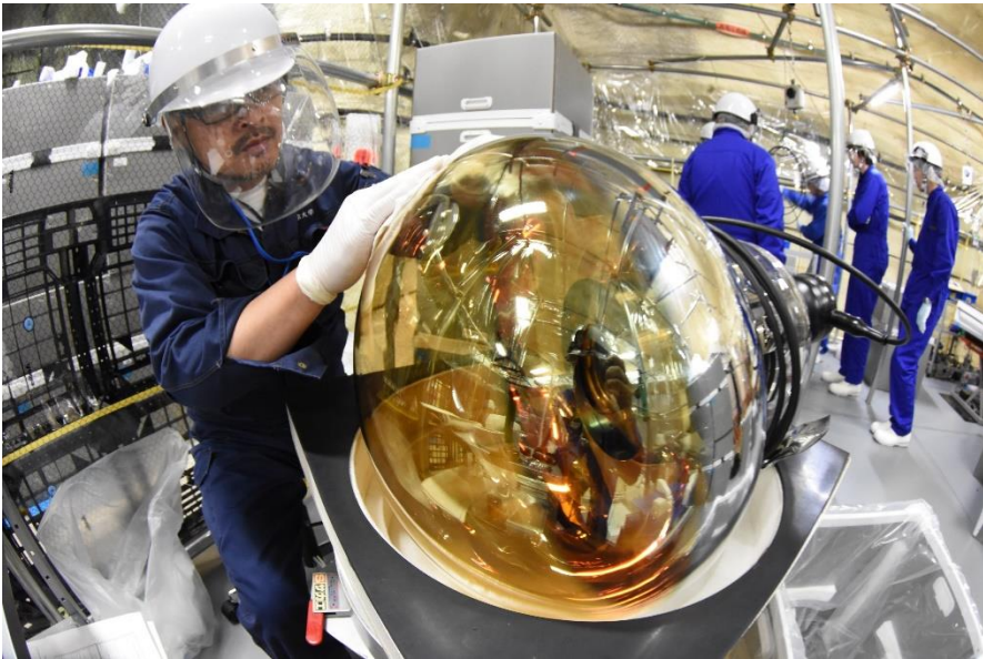
Cleaning PMT and check glass surface.
