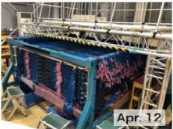
(xii) Light barrier/cables assembly
