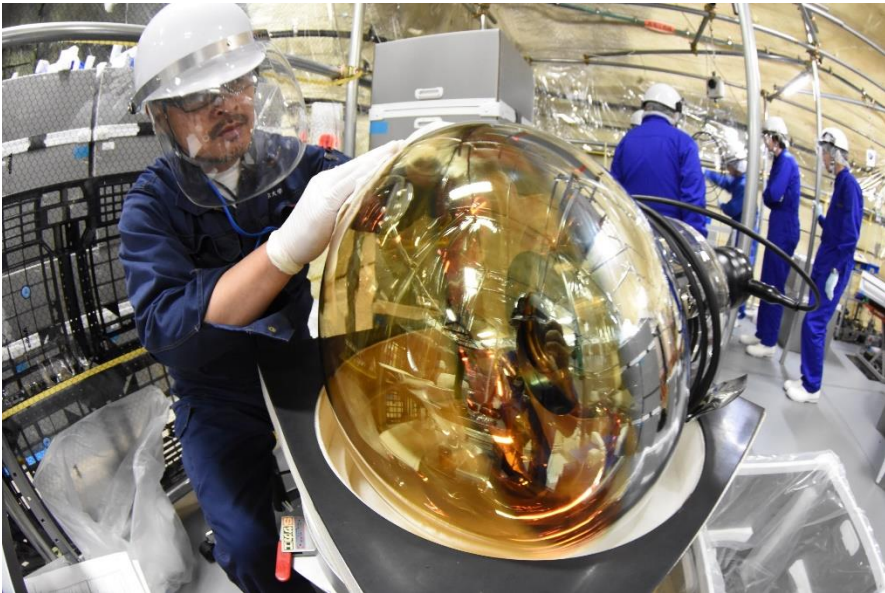
Cleaning PMT and check glass surface.
