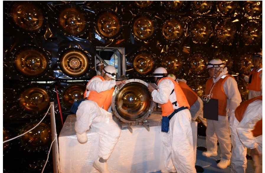
Removing bad PMT
