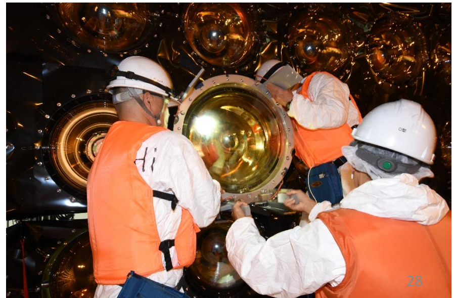
Attach new PMT
