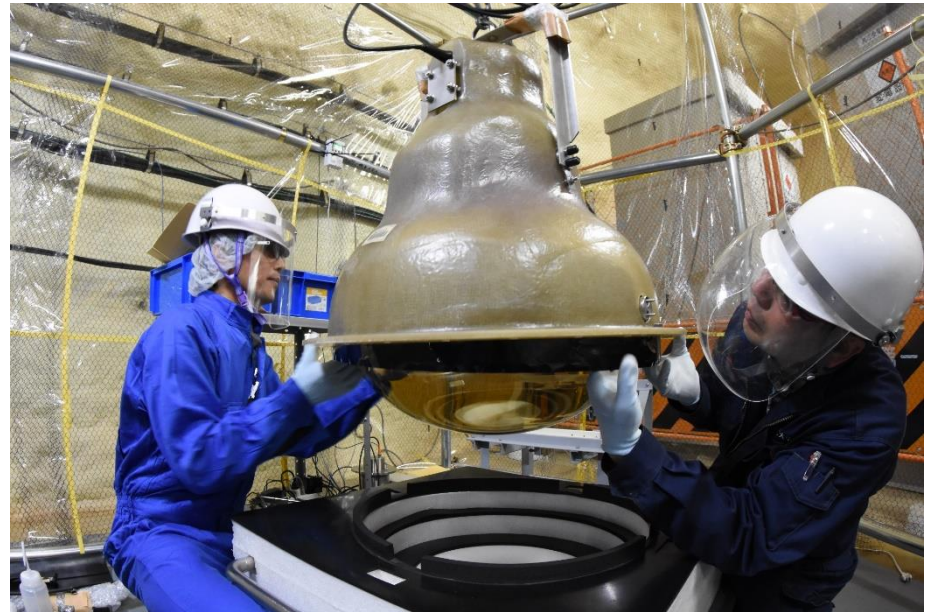
Attach PMT cover.
