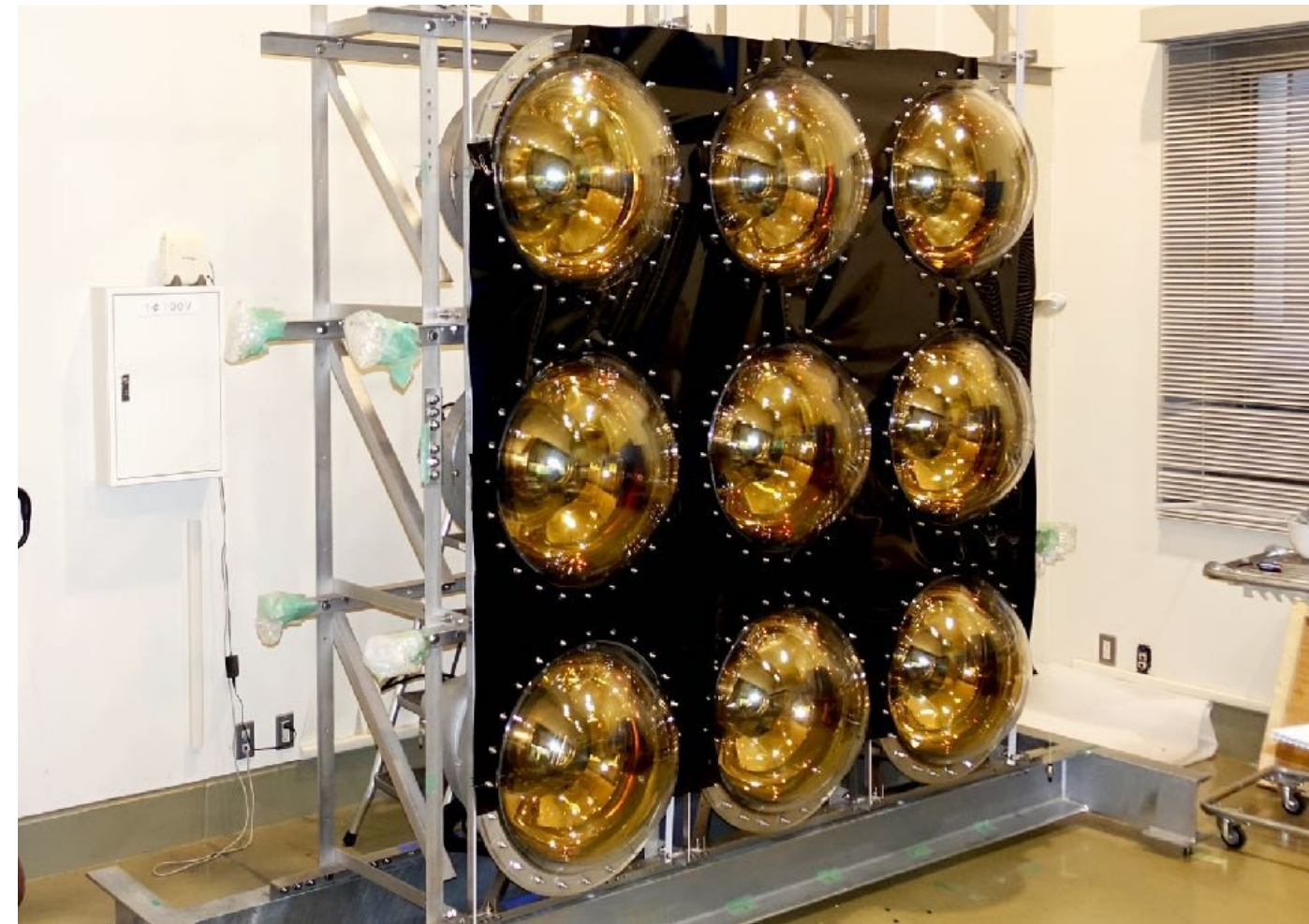
Multi-PMT module: Outer detector: PMT+WLS plate
