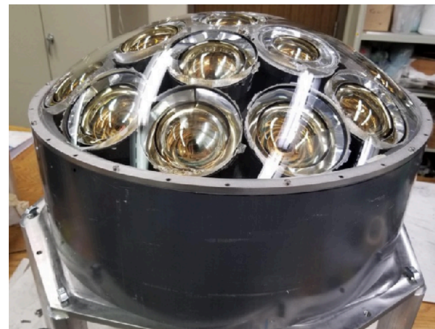
Multi-PMT module: Outer detector: PMT+WLS plate
