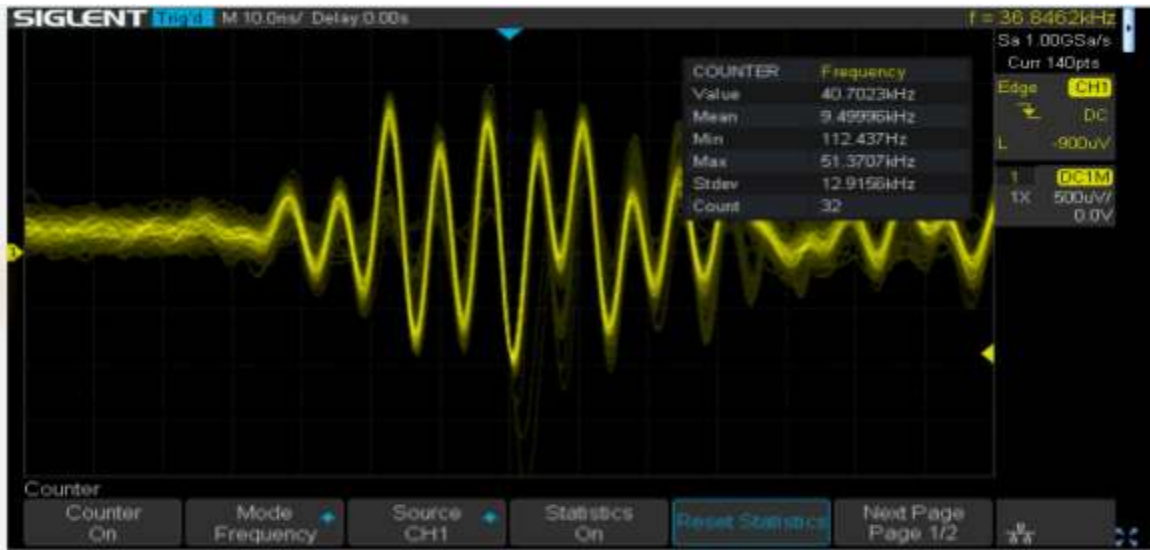
Fig 3: PMT noise rate at -0.9mV with DC power supply on
