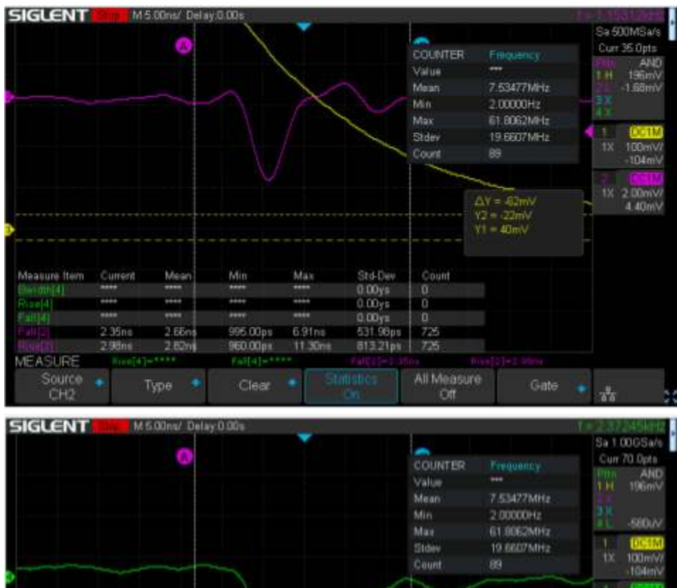
Fig SEQ fig \* ARABIC 5: rising and falling time in two separate channels. The upper for channel 2 and the lower for channel 4
