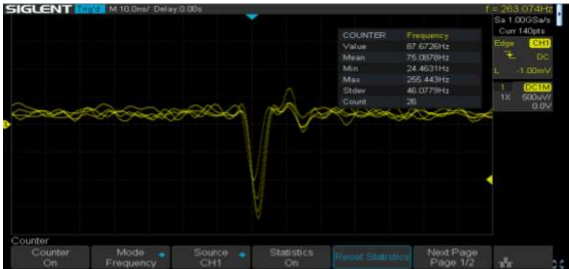
Fig 4: PMT noise rate at -1mV with DC power supply on
