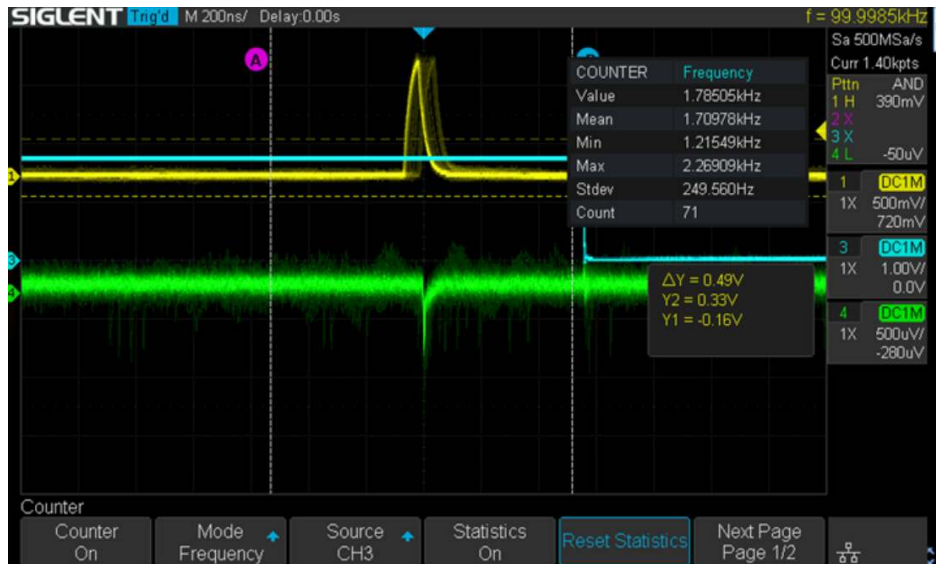
Figure 9: SiPM signal (green) and reference signal (cyan)
