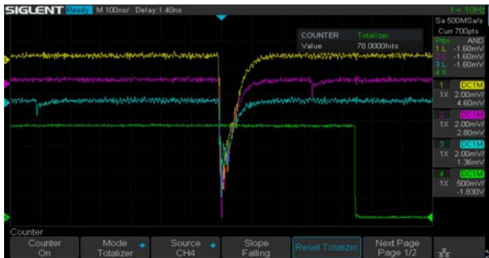
Figure 20: The muon signal coming from the three plastic scintillators
