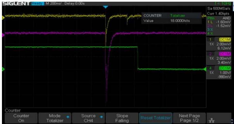
Figure 19: The muon signal coming from the two plastic scintillators
