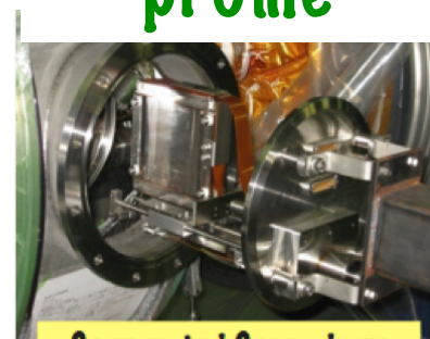
Segmented Secondary Emission Monitor (SSEM)
