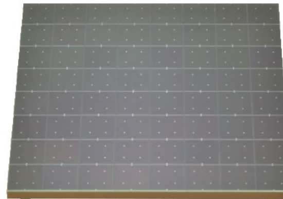
MPPC array for the ASTRI gamma-ray astronomy project • 8x8 ch. (7x7mm/elements) • High sensitivity for Cherenkov light
