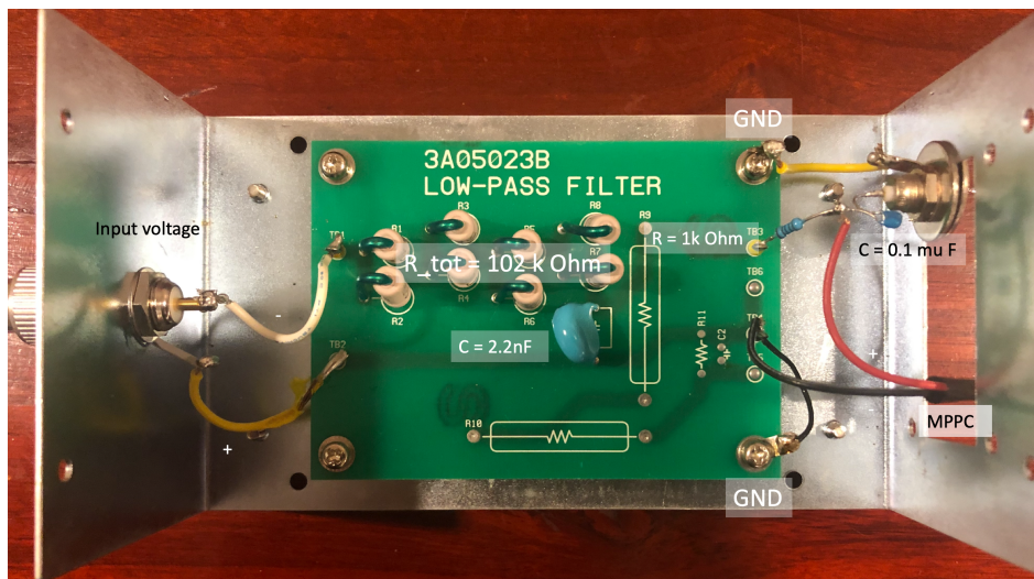
Figure 2.2: MPPC practical readout circuit
