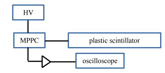
Test MPPC first generation: HV 70V Amplify 1 times Observe cosmic ray muon
